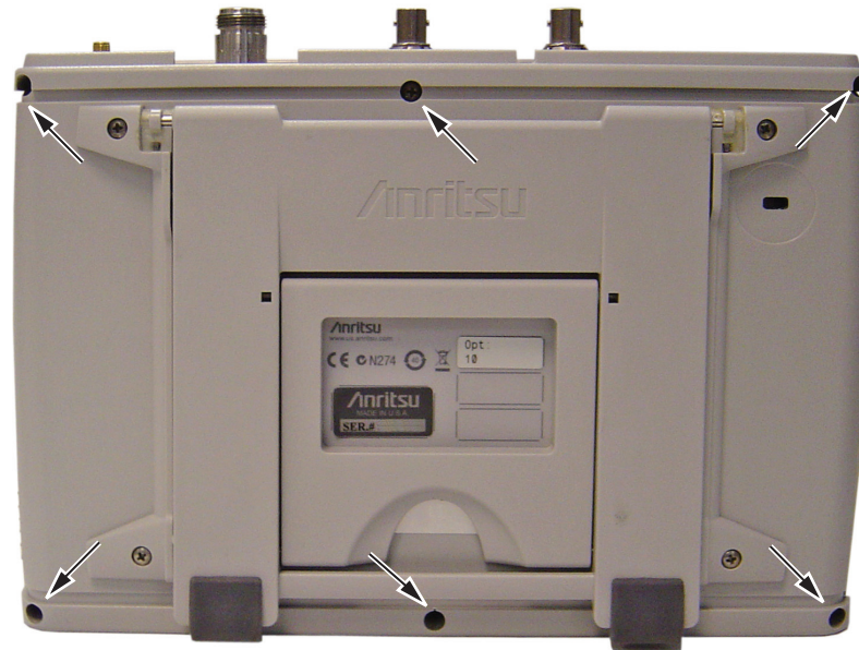
Figure 4-16. Remove the Six Screws
