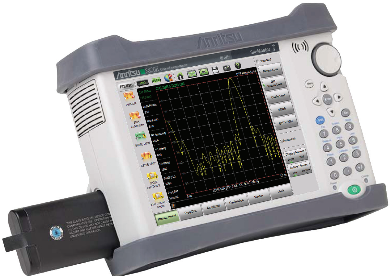
Figure 3-2. Battery Insertion and Removal
